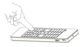
2. Aim the device's infrared LED at your original remote control's infrared LED in parallel alignment (PS: the relative distance no more than 7 cm). Press one key in Area A, the blue indicator light will start to flash, this indicates it entered the receiving Infrared status.
